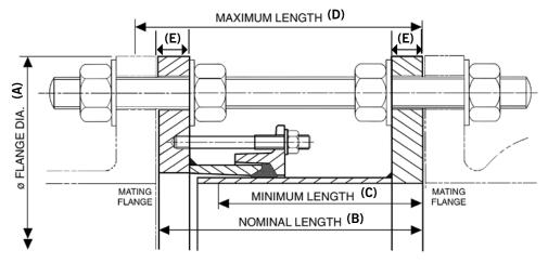
**Note:** Maximum Longitudinal Adjustment = Maximum Length – Minimum Length
